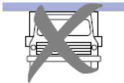
Load too large for vehicle, projecting too far from sides
