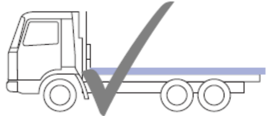
Vehicle correct size for load, rear projection within permitted limits
