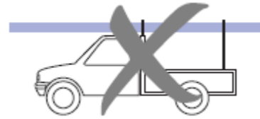
Load too large for vehicle, projecting too far from front and rear
