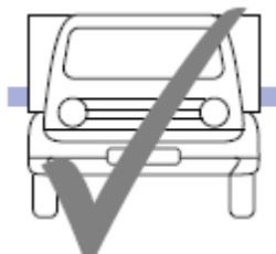
Vehicle correct size for load, side projection within permitted limits
