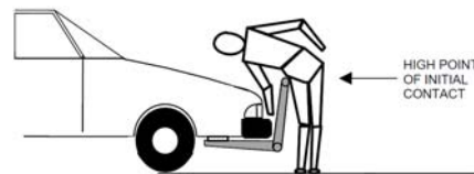
Figure 2. Pedestrian collision with a poorly designed bull bar Pedestrian pivots about the high contact point, with increased risk of spinal, pelvic and head injuries
