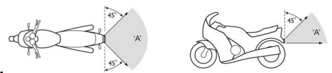
The number plate must be visible from 20m at all points within the arcs marked 'A'
