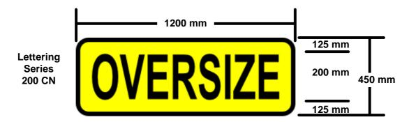
A warning sign on a vehicle/combination must be mounted:
